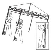
5) Lift each leg until the button snaps into the first hole.
