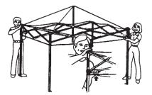
4) Push plastic socket over button on leg to tension roof.
